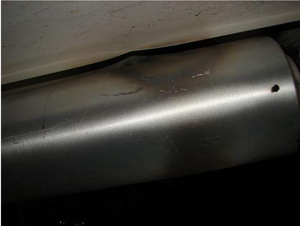
A hole, burned through the outer wall (aluminum) of the silencer as I discovered after the landing (80 flight hours in the log).
