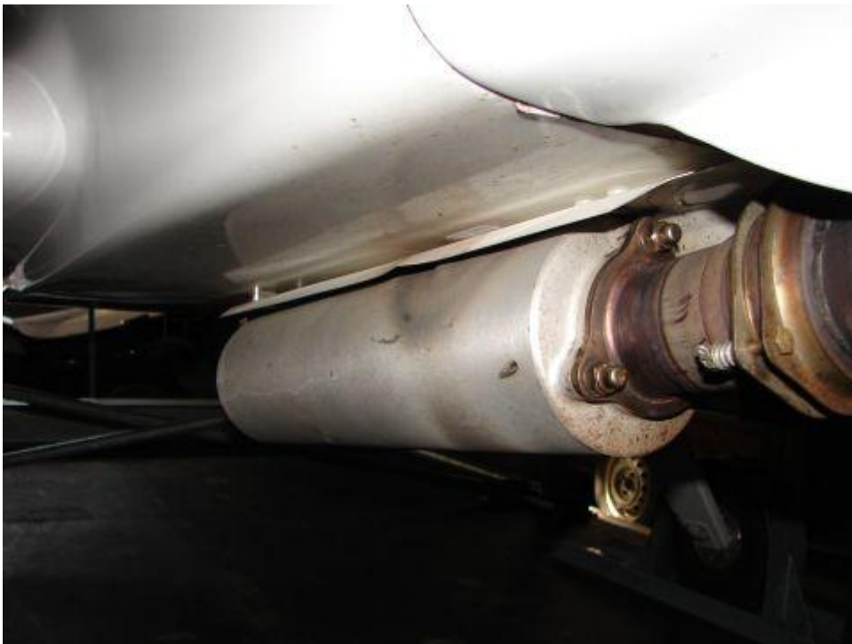
The heat-protection-shield performed well. Though, I need a better solution.
