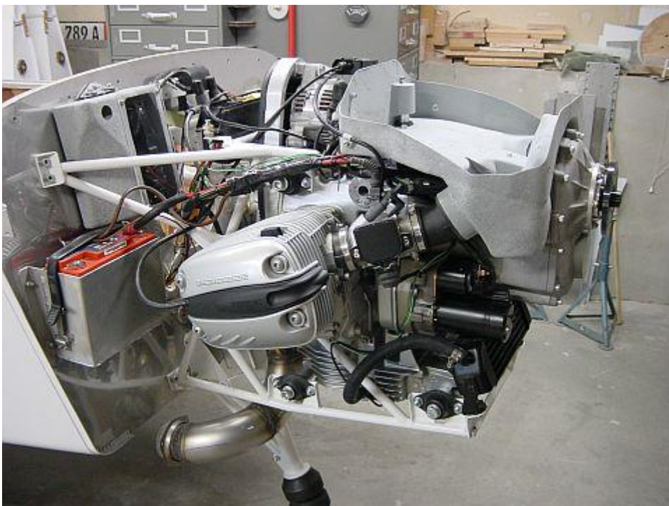
Filter Housing with original BMW inlet ducts (black)
