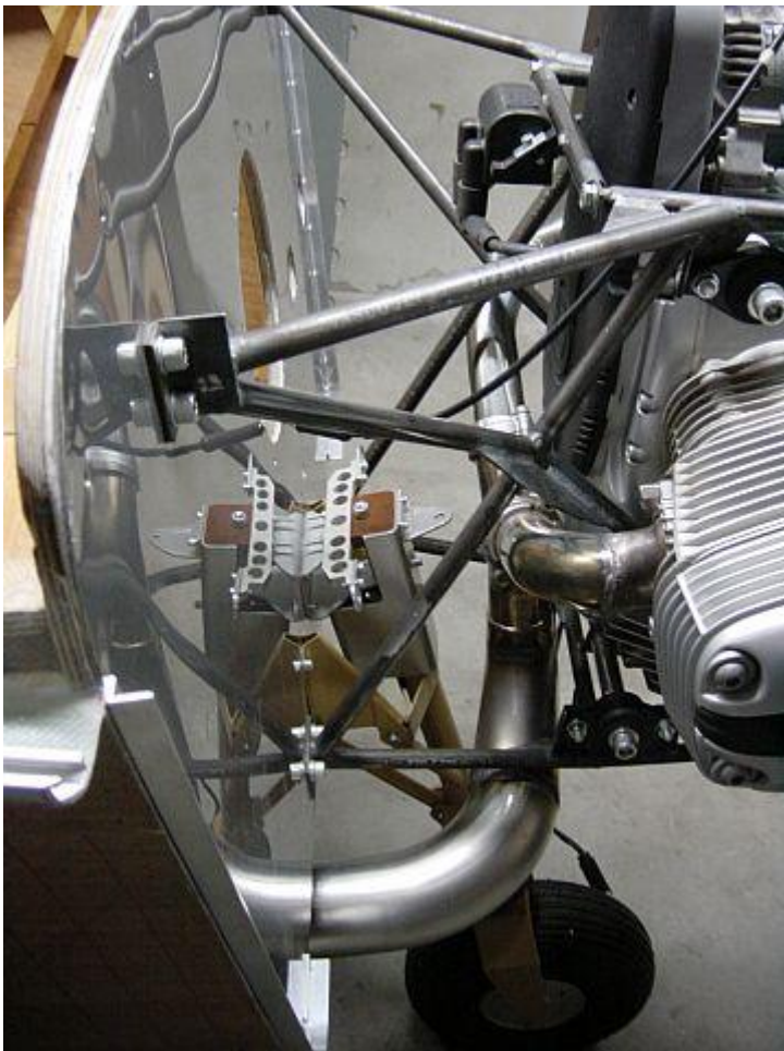
The 75 mm (3") elbows will serve as a kind of first stage pod
